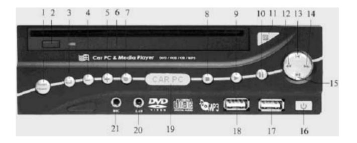
Please Note: The silvery key on the panel is provided for operation with etDVD multimedia playing software. While in the PC mode the POWER key is the only key which will function. With the exception of the POWER key, the following key description targets the etDVD multimedia software.
