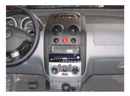
Above photo shows installed Car PC after unit has been installed into dash. Snap detachable plastic front panel frame into place. See photo and description 4.4.
