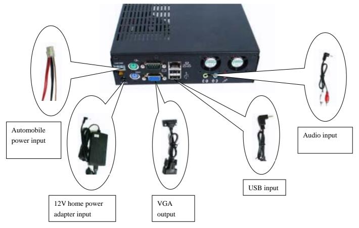
Note: if operated in a home environment, use the home power adapter (provided) input instead of the automobile power input. Other connections remain the same.
