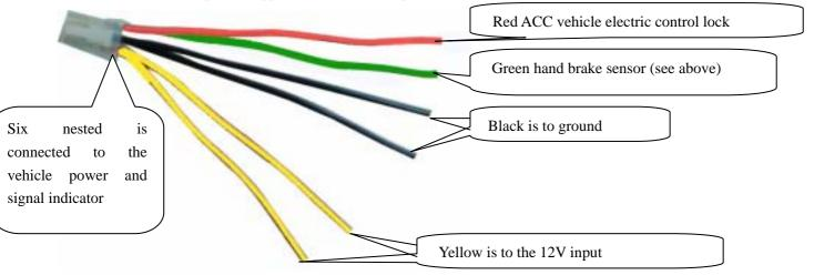
4.3 Other signal port connections, depending on users' external equipment requirements:
