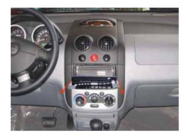
4. Remove the unit from the vehicle along with all furnished cables
